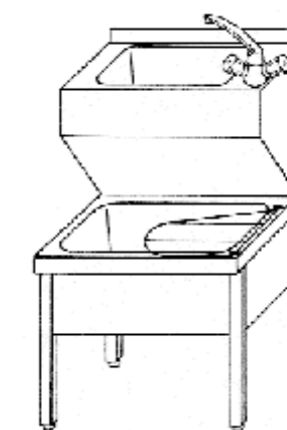
hand basin and spiller EMAX-7000 570x620x900 upper basin: 430x280x130 bottom basin: 500x500x250 EMAX-7000 520x620x900 upper basin: 430x280x130 bottom basin: 500x500x250
